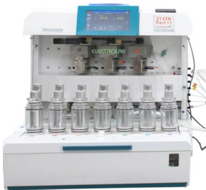
Figure 4 Basic unit (cell unit and pump unit) sample collection is completely manual
